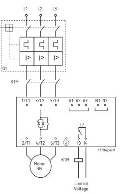
Example 3 – MCD 201 installed with circuit breaker, overload and line contactor.
